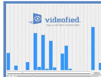
The video frame shown above is of a Videofied message being transmitted across many different frequencies (spread spectrum). If there is interference or "jamming" on a frequency, the system works around it to find an open lane to transmit the message/video of the alarm.
